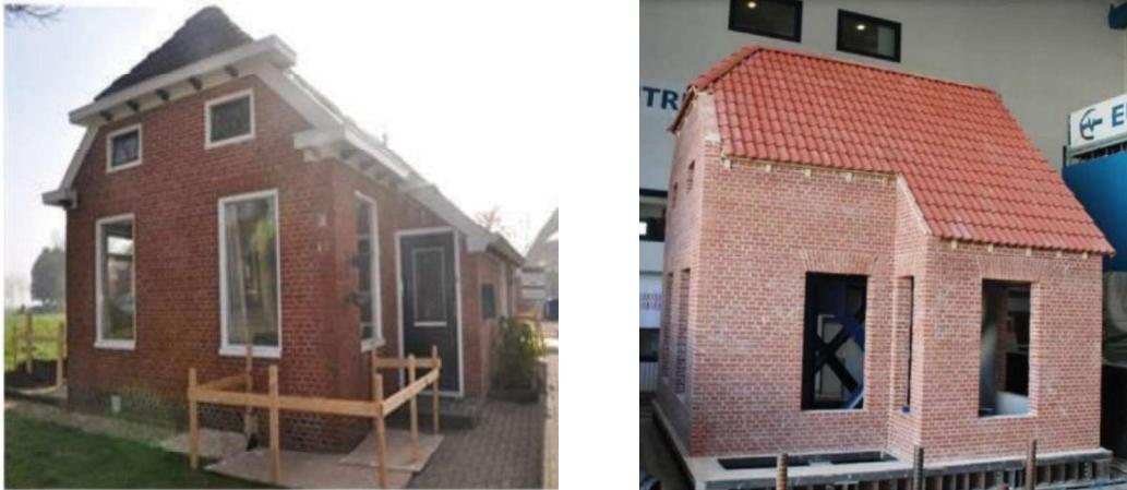
**Figure 1: Buildings with construction details similar to those adopted for the shake-table test specimen (from [2]), and actual specimen tested at the laboratory of Eucentre (from [5]).**
