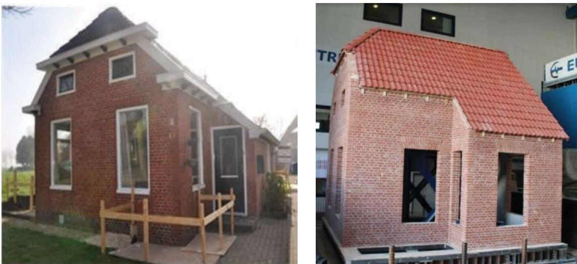
Figure 1: Buildings with construction details similar to those adopted for the shake-table test specimen (from [3]), and actual specimen tested at the laboratory of EUCENTRE (from [5]).
