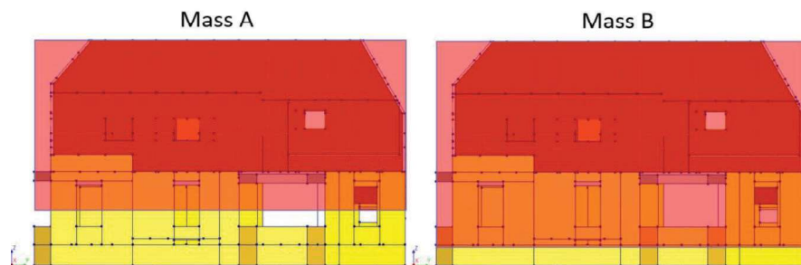
Figure G.8 Considered effective masses (portion of the house highlighted in red) for Damsterweg 37: Mass A (53.3 ton, left) and Mass B (99.1 ton, right). Adapted from Annex H.
