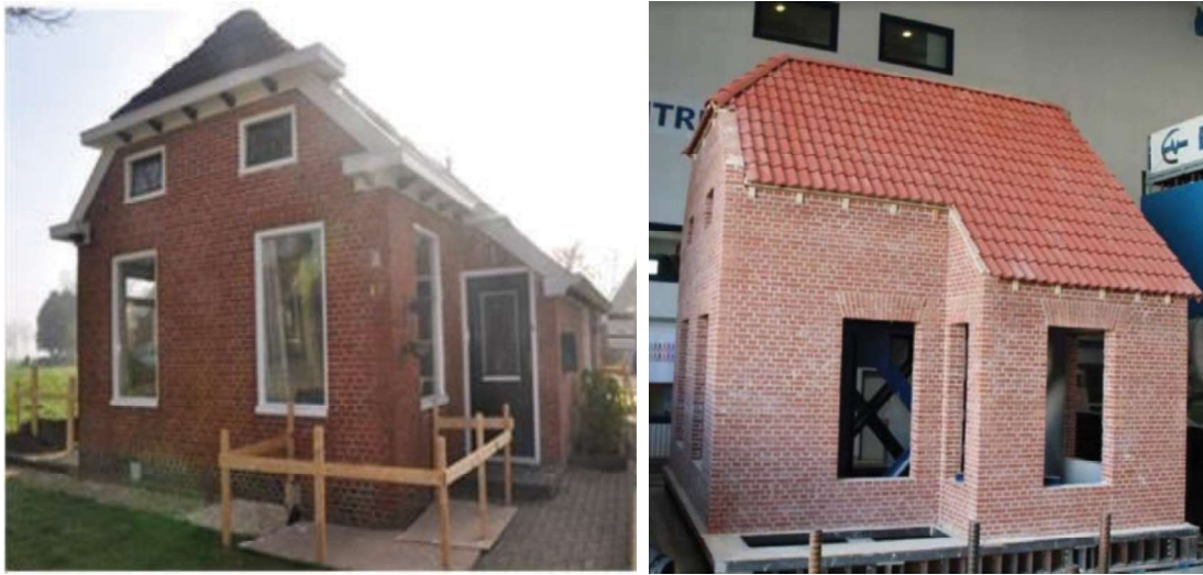
Figure 1: Buildings with construction details similar to those adopted for the shake-table test specimen (from [2]), and actual specimen tested at the laboratory of Eucentre (from [6]).
